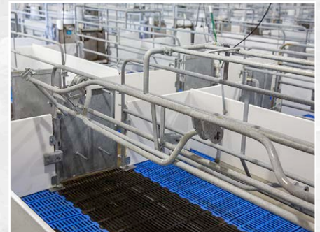
Flip Up Panel for Easy Access to Sow from Side
